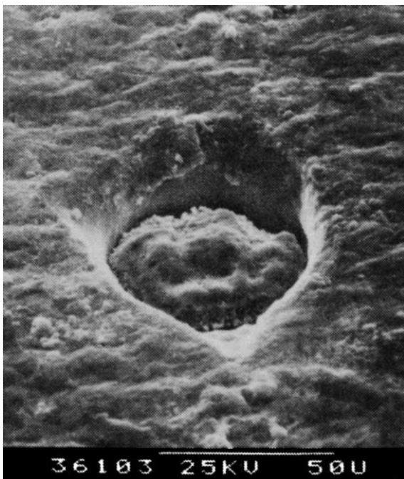
Fig. 9. SEM micrograph of LACE formed surface morphology of Ni (80%)–Fe (20%). Etching by CCl_4 at 100 Torr was driven by a 120 s pulse, focused Ar laser beam (taken from Ref. [23]). This picture shows that deeper etching has occurred at the edges—possibly due to thermally driven inhomogeneities within the CCl_4 that result in variations to the initially Gaussian beam profile.
